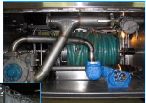
700 Series meter, DMP pulse transmitter and register on a delivery vehicle...
